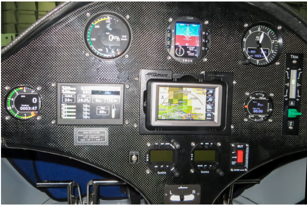
Figure 3: Avionics of Pipistrel Alpha trainer.
