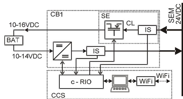
Fig. 2: Diagram of controlled power controller CB1.
