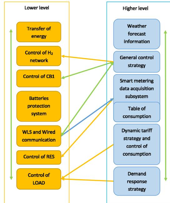
Fig. 4: Structure of the SEM control and data acquisition.
