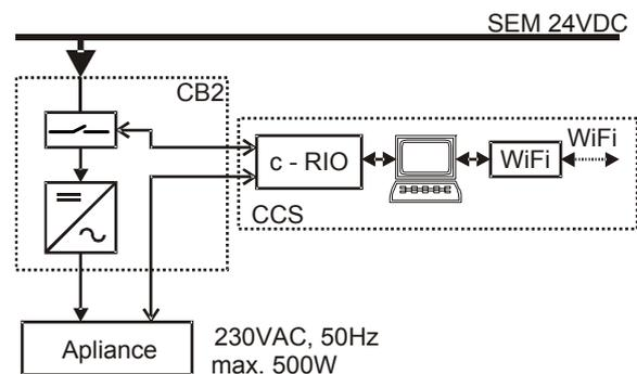
Fig. 3: Control unit CB2 of appliance.
