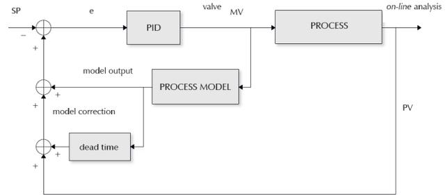
Figure 9: Model-based control scheme for dead-time compensation.
