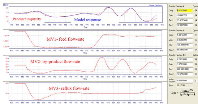
Figure 4: Multivariable control loop model identification – closed loop mode.
