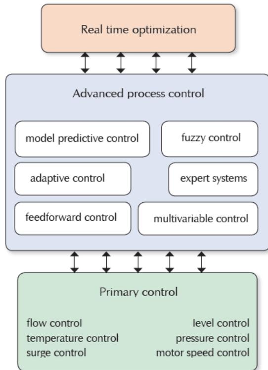
Figure 1: Process control hierarchy.
