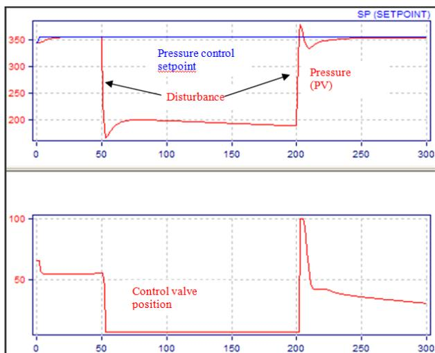
Figure 5: Optimized pressure controller in presence of disturbance.
