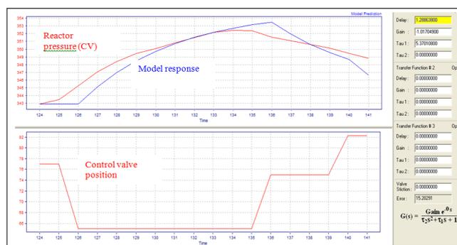
Figure 2: Pressure control loop model identification [24].
