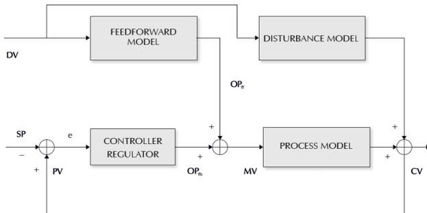
Figure 8: Feedforward control simulation and optimization scheme
