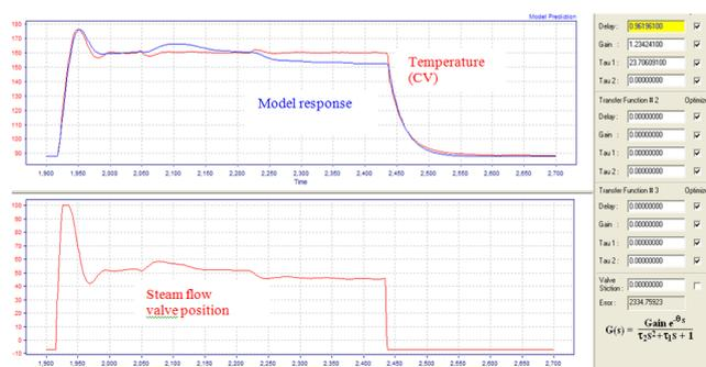
Figure 3: Temperature control loop model identification – closed loop mode.
