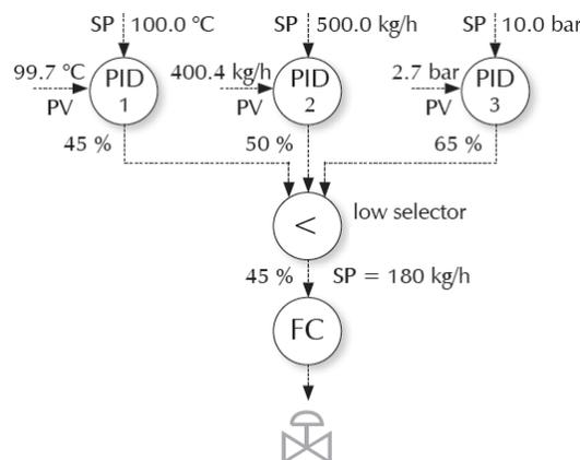
Figure 7: Production rate maximizer controllers.
