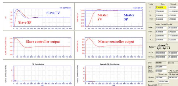
Figure 6: Optimized PID controller in presence of SP change.
